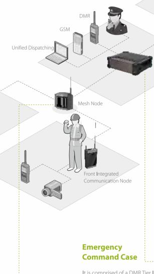
It is comprised of a DMR Tier II IP Repeater, Mesh node and Hytera SmartOne Platform, which achieves voice and video dispatching of the emergency network.
